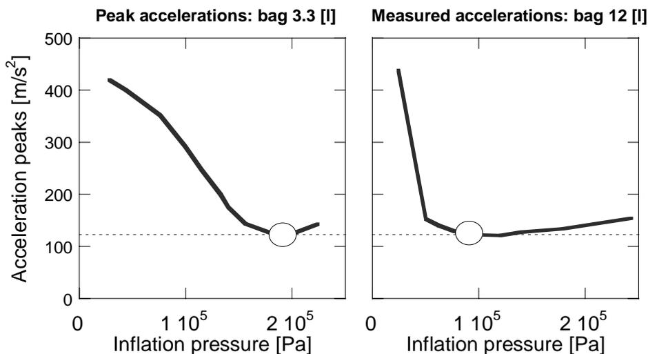
**Fig. 18 - Peak acceleration registered varying inflation pressure, for two different bags.**
