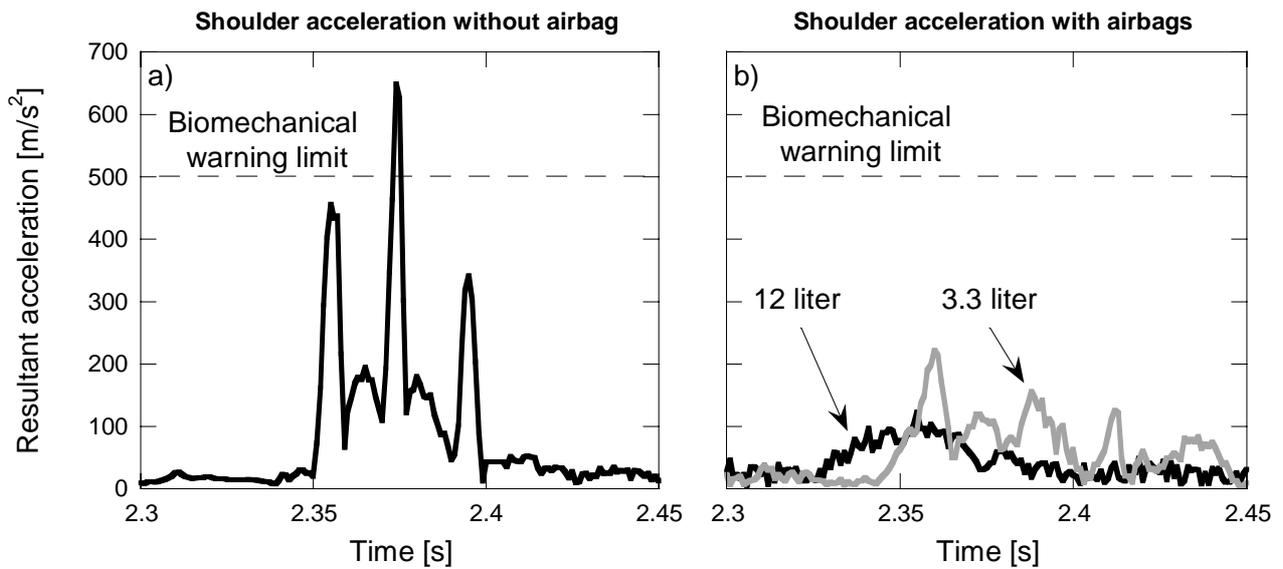
**Fig. 15 - Accelerations experienced by dummy shoulder without or with airbag**
