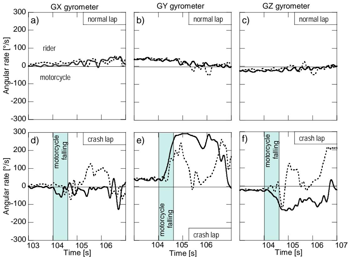
**Fig. 5 - Angular rates of motorcycle and rider recorded during a normal and the crash lap.**
