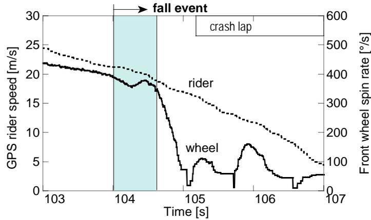
**Fig. 3 - Recorded speeds of the rider and front wheel on crash.**
