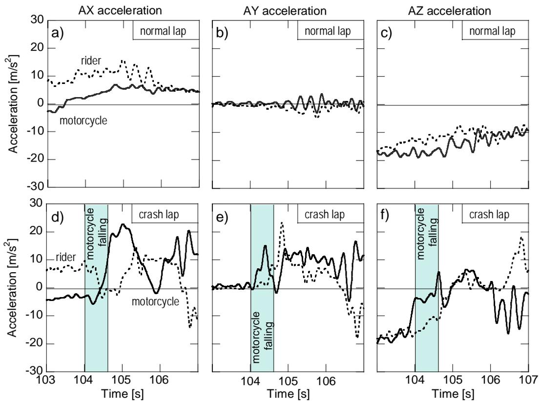
**Fig. 4 - Accelerations of motorcycle and rider recorded during a normal and the crash lap.**
