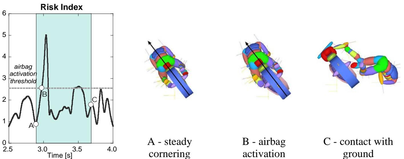
**Fig. 14 - MADYMO simulation and fall prediction of a high-side.**
