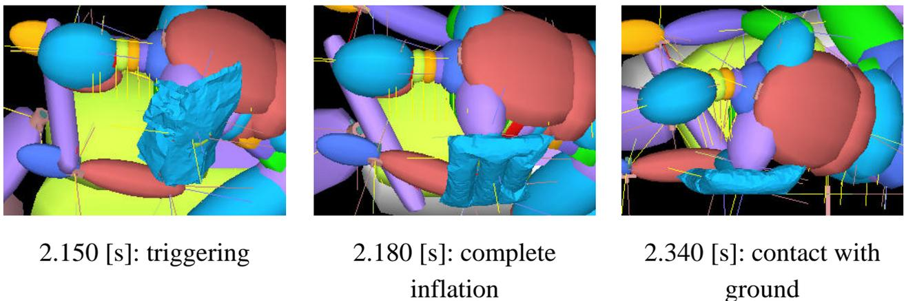
**Fig. 16 - Inflation sequence of a simulated 3.3 liter airbag system.**
