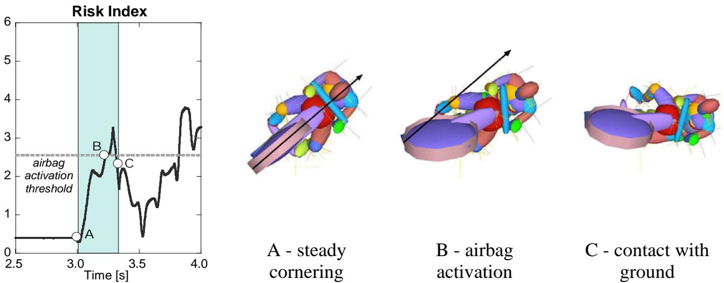
**Fig. 13 - MADYMO simulation and fall prediction of a front low-side.**
