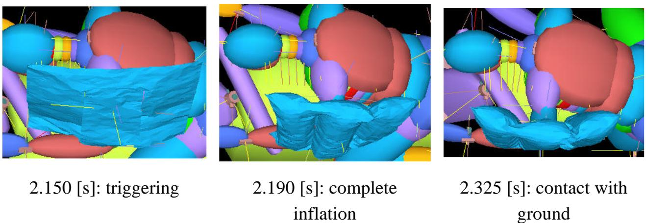
**Fig. 17 - Inflation sequence of a simulated 12 liter airbag system.**
