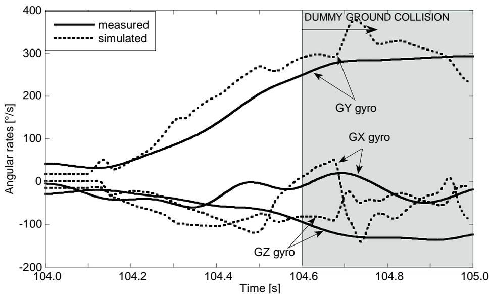
**Fig. 7 - Comparison of real data with simulation during a fall event.**
